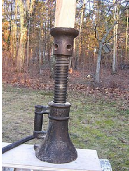
A 2.5-ton jack screw. The screw turned by inserting the bar (left) into the holes at the top, and turning it. The jackscrews turning the Pummerin must have been massive
